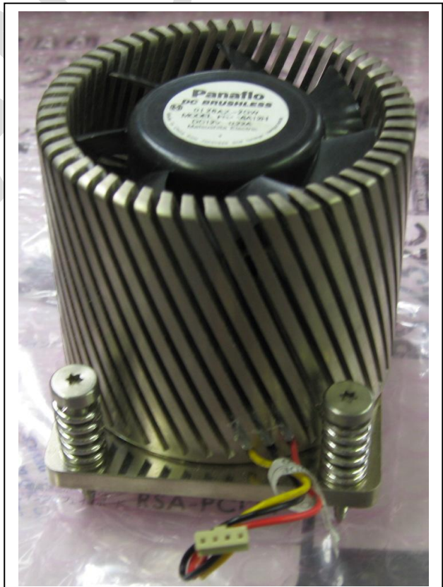
Locked CPU with four Trox screws
